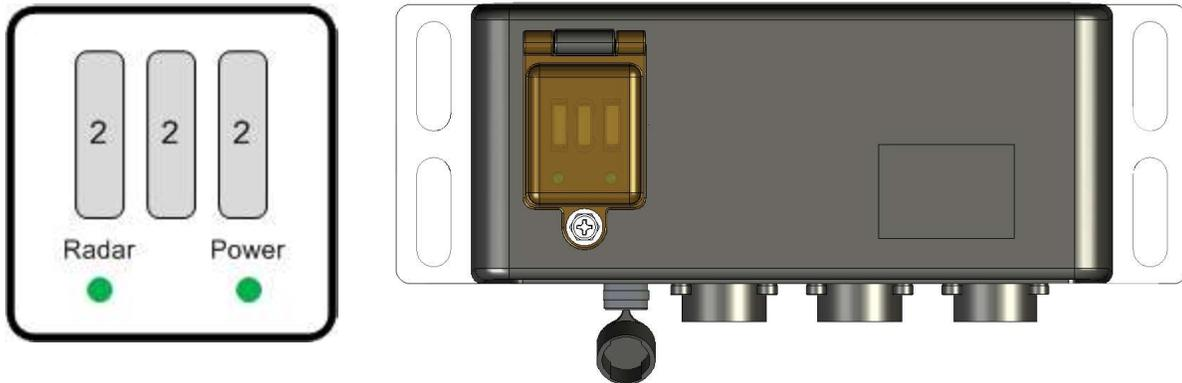
The Power LED will be illuminated green when power (+11 to +32 VDC) is applied to the controller. The Power LED will not be illuminated (off) if the 2 Amp power fuse is open or “blown”.
